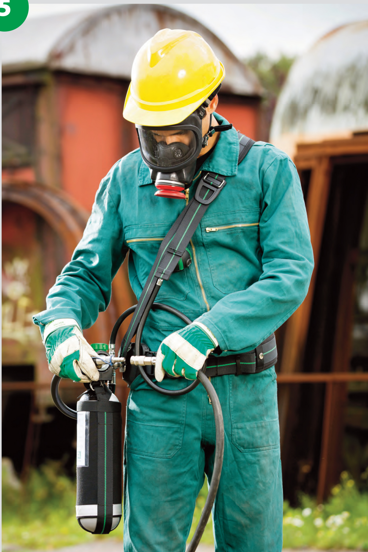
Check gauge to ensure fully pressurized cylinder. Pull on airline hose, remove protection cap and connect pigtail to airline.*
